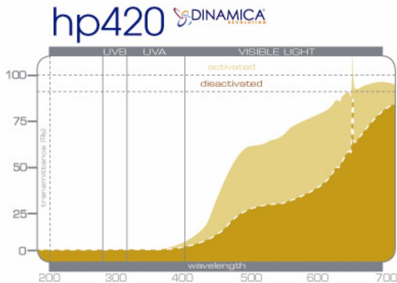
The photocromic filtering lens HP 420 protects from UVA and UVB rays (noxious light) and from the first blue light of the visible up to 420 nanometers.
