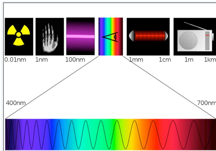
*As you can see in the figure above, visible light is just a part of the wide spectrum of electromagnetic radiations. Most part of the spectrum is invisible. The UV rays are made of invisible electromagnetic radiations with wavelength between 400 and 100 nanometres..*
