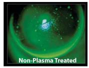
The FeelSoft plasma treatment process modifies the superficial layer of the GP lens and generates a hydrophillic surface that promotes enhanced wettability. FeelSoft plasma treated lenses will create a reduced wetting angle and can potentially increase comfort during wear.
